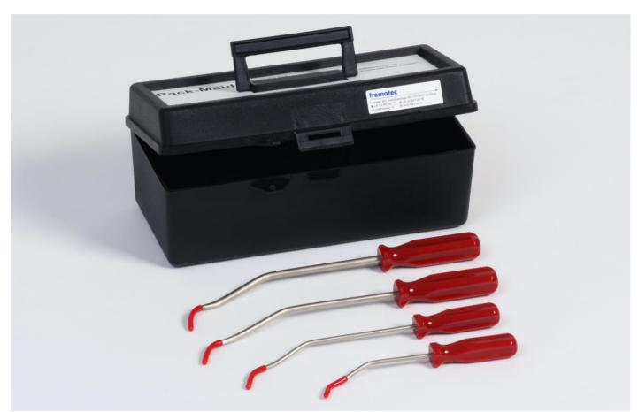
How to handle: The grooves on the handle lined up so that you get the maximum leverage from your wrist and thumb. The complex angels of the tool will help give proper penetration around the shaft and into the packing. These special tools are made of high carbon, heat treated steel.
