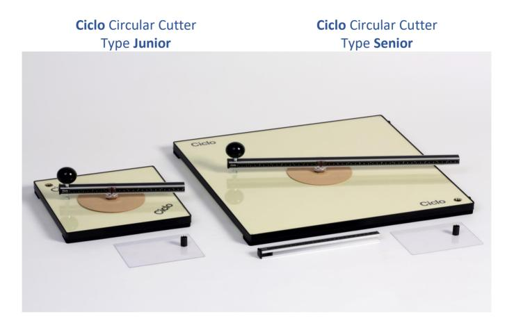
**Type Junior for :** from centre 30 up to 270mm Ø, from corner 270 up to 500mm Ø **Type Senior for:** from centre 30 up to 500mm Ø, from corner 500 up to 1000mm Ø
